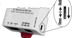
**3.** Connect both the tDS-700 and the Host computer to the same sub-network or the same Ethernet Switch, and then supply power (PoE or +12 to +48 VDC) to the tDS-700.
