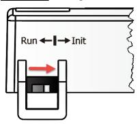
For tDS-700 series modules, the operating mode switch is set to the **Run** position by default. In order to update the firmware for the tDS-700 series module, the switch must be moved from the **Run** position to the **Init** position. The switch must be returned to the Run position after the update is complete.
