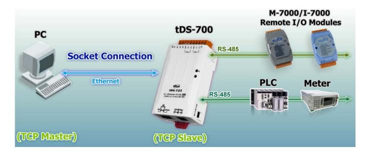
tDS-700 series module can accept the TCP connection (include raw data) directly, it also can communicate with TCP client and Serial Device in this way.
