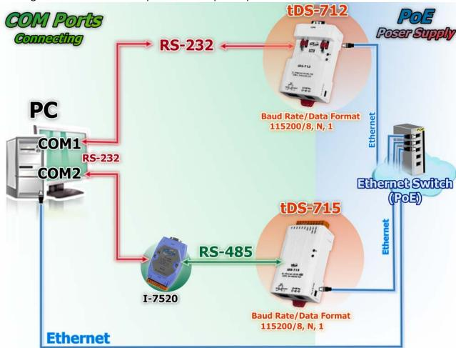
The image below shows an example of the setup for a pair-connection test:
