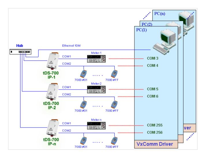
The VxComm driver controls all the details of the Ethernet TCP/IP programming technique, meaning that, with the assistance of tDS-700 and VxComm technology, your COM Port program will be able to access your serial devices through the Ethernet in the same way as through a COM Port.
